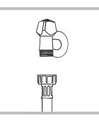
2. Connect the inlet hose by screwing it to a cold water tap using a 3/4 gas threaded connection (see figure).
